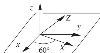
12. Write direct and inverse formulas for the changes of coordinates between system  $Oxy$  and system  $OXY$ . The second system is constructed by the composition of a rotation of  $\alpha$  around  $z$  axis and of a rotation of  $\beta$  around  $X$ .
