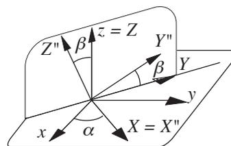
13. Write direct and inverse formulas for the changes of coordinates between system  $Oxy$  and system  $OXY$ . Note that  $Z$  axis passes through the point  $P\{x = 2, y = 1, z = 1\}$  and  $X$  axis lies on the (ground) plane containing  $x$  and  $y$  axes.
